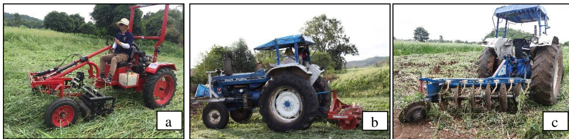
Fig. 1 (a) USDA roller-crimper, mounted on Oggun; (b) Cambodian made roller-crimper, pulled by 75-hp diesel tractor; (c) disc-pow with six discs
